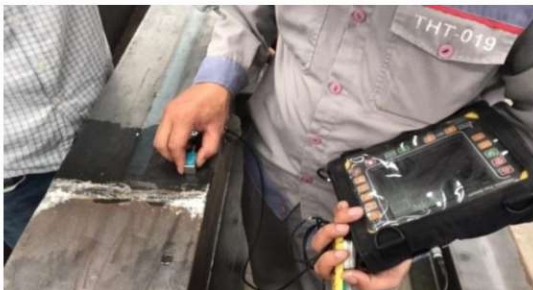
Checking butt welding and connection plate welding by Ultrasonic machine
