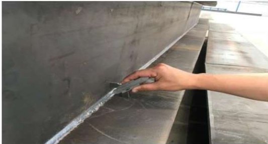
Checking butt welding and connection plate welding by Ultrasonic machine
